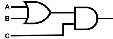
*Answer: The first gate is A OR B. With A being off (false) and B being on (true), A OR B is on (true). The second gate is (A OR B) AND C. With A OR B being on (true) and C being off (false), the second gate is off (false).*
