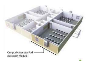
To adjust the size of the CampusMaker ModPod the two classroom module at either end can be detached and relocated to another site or school. Construction of a new exterior wall is not required as the wall and finishes are already in place. This feature minimizes the down time due to construction and disruption to the remainder of the classroom complex.
